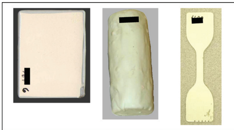
Fig. 2: Severe Wastewater Analysis Testing specimens. (not to scale) (left) coated steel panel; (middle) coated cylindrical concrete specimen; (right) molded free film sample
