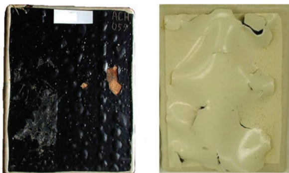
Fig. 9: Example of blistering on steel panels. Coal-tar epoxy (left) and high-build amine epoxy liner (right) following S.W.A.T. exposure.
