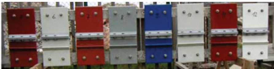
Fig. 7: Specimen design for splash zone (SZ); dimensions in mm Courtesy of the authors
