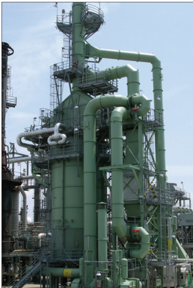
Many properties may be needed in a high-heat maintenance coating, such as color stability, surface tolerance, corrosion resistance, and high-temperature application, as on the crude oil heater unit at this refinery. Photo courtesy of Dampney Co.
