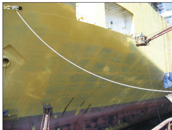
The see-through condition of the self-inspecting paint indicates on this hull that the coating has not been applied yet to the correct dry film thickness. Photos courtesy of Nippon Paint Marine Coatings Co.
