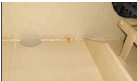
Fig. 3: Solvent-free epoxy after 8 years in service Courtesy of Van Zonderen Offshore
