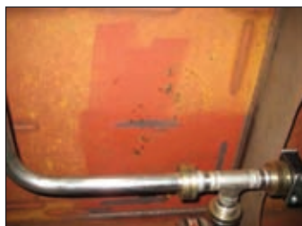
Top: Before the CO 2 cleaning Bottom: After the cleaning, even the burned shop primer has been fully removed.
