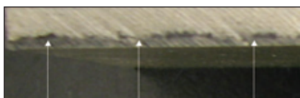
Fig. 8: 20-mil discoloration in filled, 100% solids blended amine-cured epoxy lining in total of 90+ mils
