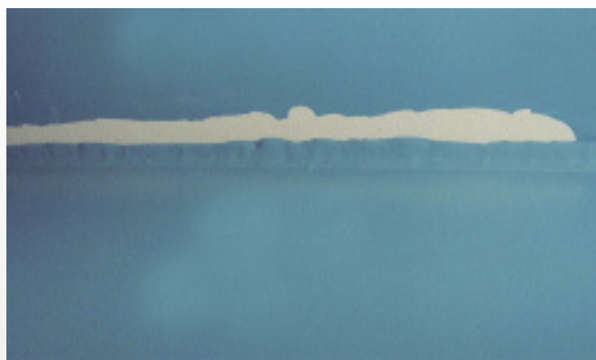
Fig. 2: X-cut testing showed poor topcoat adhesion at welds and corners.
