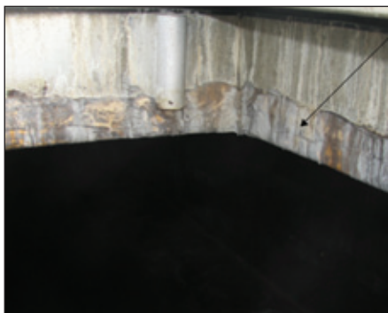
Fig. 12: Flexible, oil-modified polyol polyurethane disbonded from surfacer material
