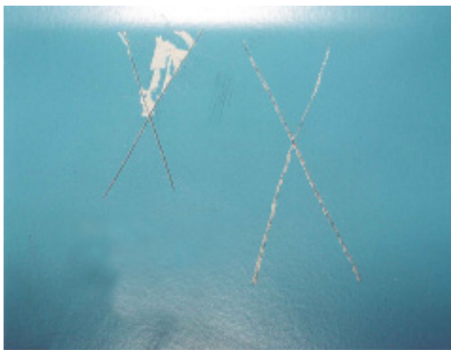
Fig. 1: X-cut for adhesion testing per ASTM D3359. Figures 1-7 courtesy of John Clayton
