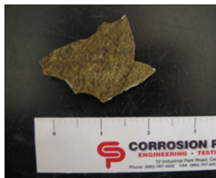
Fig. 13: Chip from disbonded, flexible, oil-modified polyol polyurethane lining
