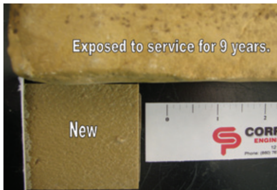
Fig. 6: No obvious sign of film degradation in highly filled, blended epoxy amine-cured mortar
