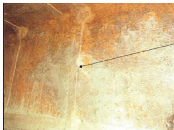
Fig. 2: Failed seam weld was the only sign of degradation from permeation on anchored PVC sheet.
