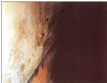
Fig. 9: Localized corrosion craters at pinholes in 100% solids, unfilled, blended amine-cured epoxy lining
