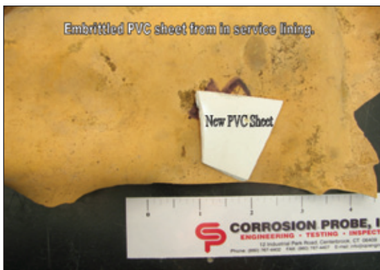
Fig. 3: Embrittled fully bonded PVC sheet from in-service lining
