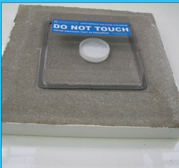
Concrete panel used for the calcium chloride test. Photos courtesy of the author
