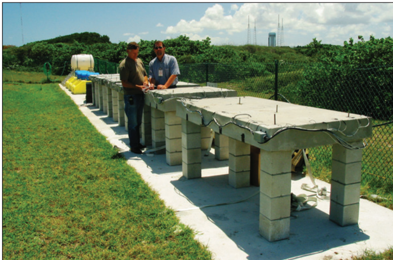
Scaled-up test/demo reinforced concrete slabs for Liquid Applied Galvanic Coating Courtesy of NASA
